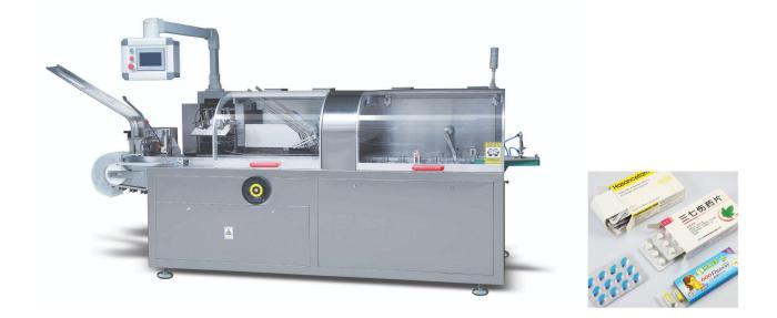
This model is suitable for inserting blister packages into cartons. It has a range of applications and is suitable for ALU-PVC blisters, ALU-ALU blisters and other similar products.
